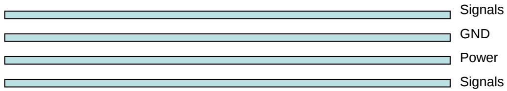
Figure 10: Typical 4-layer PCB construction
